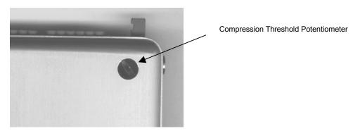
When turned fully clockwise, the compressor is turned off and the recording is completely linear. Under these conditions, the global gain of the SNST-R through the input and output cables (SCLST-R and SCUCSTR) is unity.
