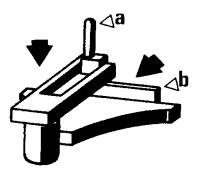
To rewind, turn the handle clockwise without pressing downwards so that the reels turn freely. Once the operation is completed, centre the handle between the two reels, disengage it by pressing (b) and push back into place; fold down (a).
