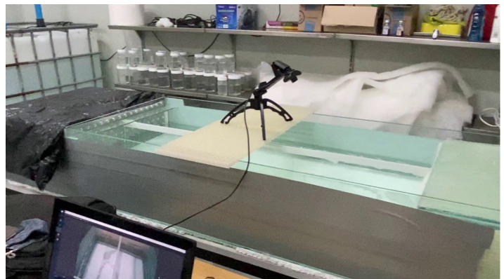
Figure 8. Chamber developed by Yansivan Kisten to test the attraction of young fishes to potential chemical cues from different sources
