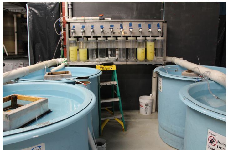
Fig. 19. UWSP NADF bell jar incubation system with collection insert tanks
