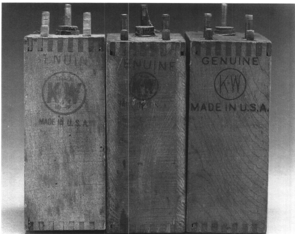
Photo 35: Three differently marked K-W coils. These coils were supplied to the aftermarket retail trade for Model T parts in the millions. Note that the studs used to attach the points to the top of the coil are threaded from top to bottom. This is characteristic of coils manufactured by K-W Ignition Co.
