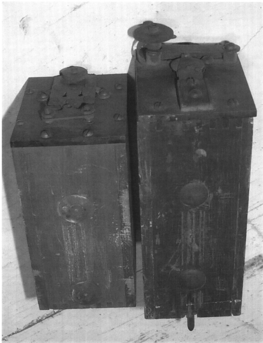
Photo 11: Jacobson and Brandow coils used in 1910, 1911 and 1912. The taller of the two coils was used in 1910 and 1911. The shorter coil saw limited use in 1912.
